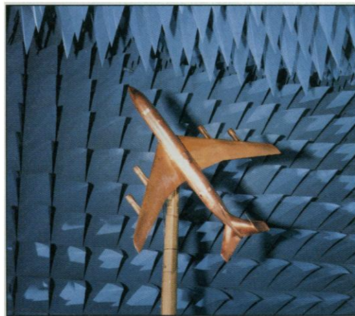
Final flight. Scientists at Rome Lab, facing consolidation, measure electromagnetic effects on air frames.
