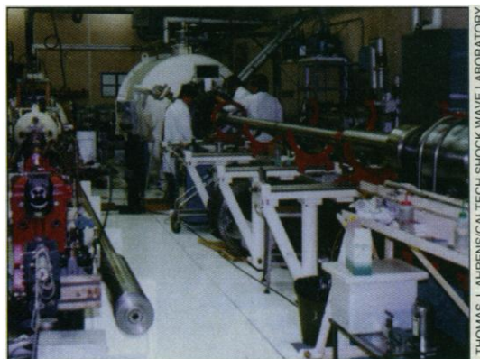
Big guns. Shock waves produced in high-speed guns can melt iron under conditions of Earth's core.
