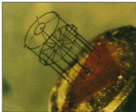
**Fig. 1.** Three-dimensional free-standing alumina microstructure fabricated directly from the vapor phase by LCVD. The fiber segments, each having a diameter of 20  $\mu\text{m}$ , were continuously formed and joined in this two-laser LCVD process. [Reprinted from (1) with permission; copyright, Elsevier Science]
