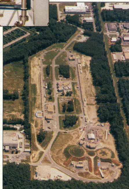
Hidden advantage. CEBAF's tunnel follows the racetrack outline visible in the photograph. Niobium superconducting cavities (top) accelerate the continuous electron beam.
