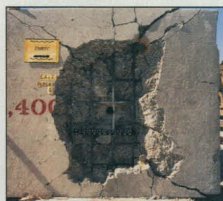
Bunker mentality. Hypervelocity projectile for attacking underground facilities passes through reinforced concrete block; entry hole is shown in the photograph above, left, and exit hole above, right.
