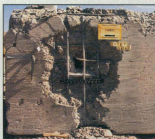
Bunker mentality. Hypervelocity projectile for attacking underground facilities passes through reinforced concrete block; entry hole is shown in the photograph above, left, and exit hole above, right.
