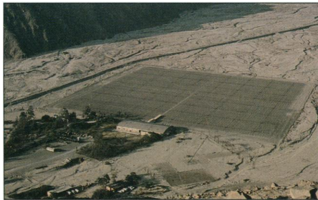
Joint venture. A field of radar antennas at Jicamarca, Peru, probes the upper atmosphere. Peruvian geophysicist Ronald Woodman directs the installation, which is funded by the United States.
