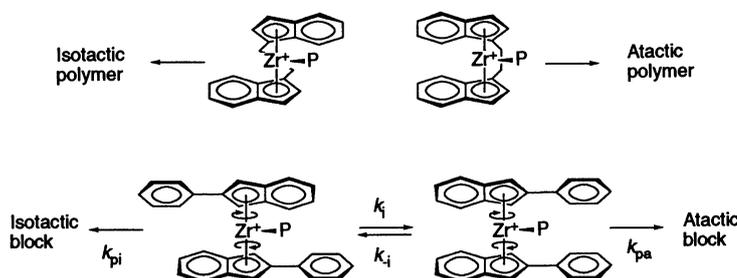
**Fig. 1 (top).** Isotactic, atactic, and stereoblock polypropylene (17). **Fig. 2 (middle).** Stereorigid *ansa*-metallocenes for the production of isotactic and atactic polymers.
