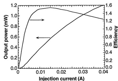
**Fig. 5.** The output power and the external quantum efficiency versus the injection current in a Nichia InGaN blue-green double heterojunction LED under continuous-wave conditions up to 40 mA.
