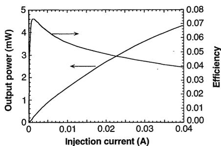
**Fig. 6.** The output power and the external quantum efficiency versus the injection current in a Nichia InGaN blue double heterojunction LED under continuous-wave conditions up to 40 mA.
