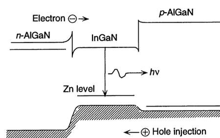
**Fig. 1.** Conduction and valence band edges of a  $pn$  double heterojunction InGaN-AlGaIn LED under injecting conditions.
