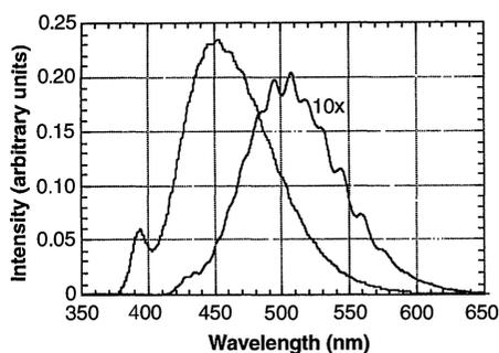
**Fig. 4.** Light output spectra obtained at 30 mA for a blue and a blue-green Nichia GaN *pn*-junction InGaN double heterojunction LED. The response of the blue-green LED is amplified 10 times.
