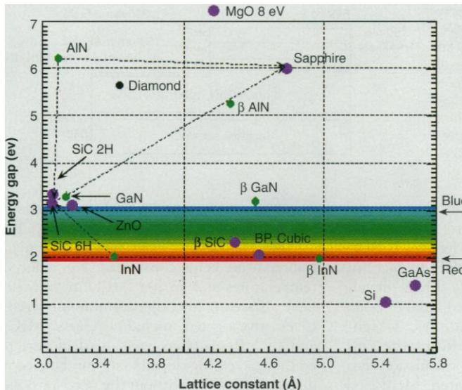
**Fig. 3.** Energy gap versus lattice spacing for wurtzite and cubic nitrides and some of the substrates on which epitaxial growth have been commonly accomplished. The color bar is not representative of the CIE diagram.
