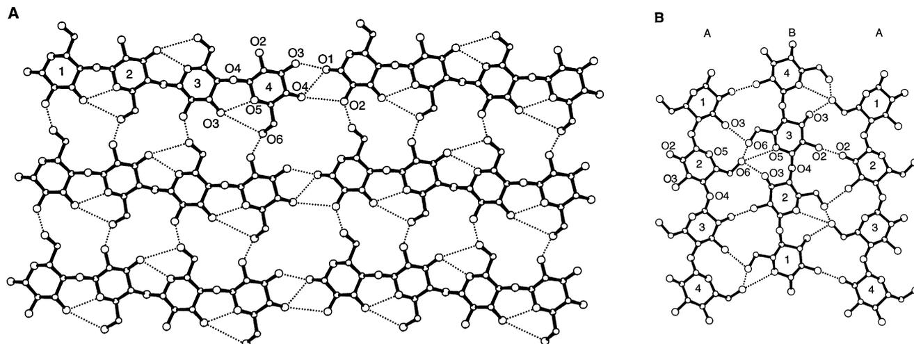
**Fig. 2.** (A) Description of the sheets of parallel molecules (A or B in Fig. 1). Dotted lines indicate short O...O contacts that are probably hydrogen bonds. The intermolecular hydrogen bonds involving O1 connect adjacent molecules in the  $c$  direction to form "pseudopolymeric" cellulose II. (B)
