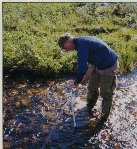
An extreme stream. Graduate student John Morrice loads a Toolik tributary with a dye to map stream flow.
