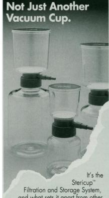
and what sets it apart from other vacuum cup devices is the low-protein binding, low-extractable Durapore® membrane. This membrane provides up to 99% total protein recovery, it won't cause alterations in protein structure and function, and it's designed to be biocompatible with cell cultures.
