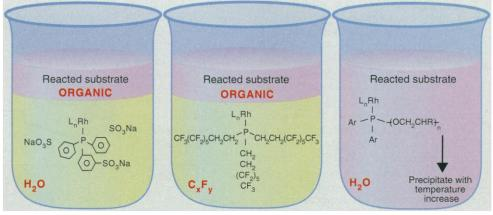
Phosphines that facilitate separation of homogeneous rhodium catalysts from product-containing phases. Adducts of the sulfonated phosphine (left) and fluorous phosphine (middle) exhibit mark-edly higher solubilities in aqueous and fluorocarbon phases, respectively. Alternatively, adducts of some special phosphines show decreased solubilities at lower or higher temperatures (right).
