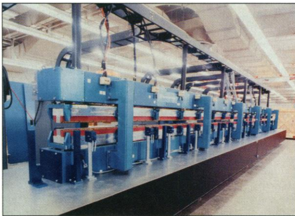
Big wiggler. This laser magnet, built for Boeing under an SDI contract, is being shipped to Brookhaven.
