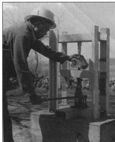
"One of the problems when looking for fossils in a hard calcified matrix is that the specimen often has to be broken, in order to discover that it is there. For this reason, a clean, predictable break is very desirable, so a machine was made . . . to ensure such breaks in blocks of Swartkrans breccia," shown here being used by Absalom Lobelo, 1968. [From Swartkrans ]
