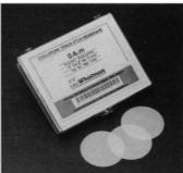
sized pores over the entire surface of the membranes. These "true pore size microporous screens" are available for collection, recovery, and analysis of a wide variety of particulates from 0.1 to 12 μm. The polycarbonate and polyester membranes can be used in air monitoring, nucleic acid studies, blood filtration for analysis of red blood cells, and wet chemical, spectroscopic, microscopic, and microbial analyses. Whatman. Circle 145.
