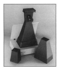
top of the hood, which provides a darkroom effect. A variety of transilluminators can be selected from, including multiple wavelengths in one unit, white light and ultraviolet in the same transilluminator, or white light only. UVP. Circle 142.
