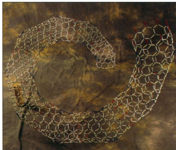
Fig. 2. One helix turn of a coiled tubule made of the same segments as in Fig. 1 except that each segment is rotated by a fixed angle with respect to the previous segment. Hence, the line connecting the opposed 5-7 rings has a rotated azimuth on progressing along the helix. [Figures courtesy of A. A. Lucas, Facultés Universitaires Notre-Dame de la Paix, Namur, Belgium]
