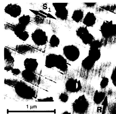
**Fig. 1.** An SFM image of a rubbed nylon layer that was also scratched. The picture was acquired at a tip loading of about  $10^{-9}$  N. The rubbing direction is marked by arrow R. The area in the top left corner shows scratches made by the SFM at a load of  $10^{-7}$  N. The scratches made in forward and backward direction are marked as arrows S<sub>1</sub> and S<sub>2</sub>, respectively.
