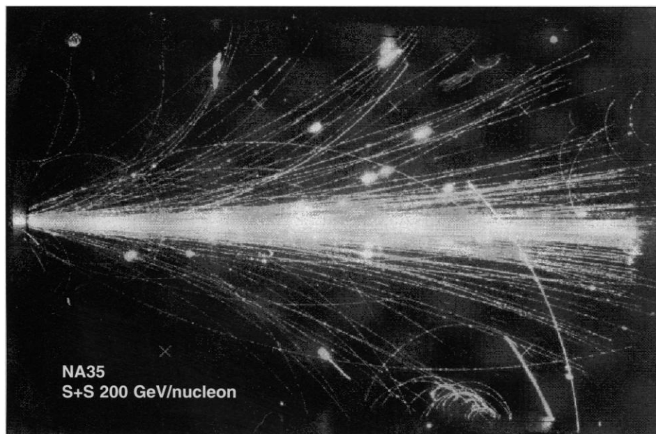
The main event. Streamer chamber photo of a single 200-GeV-per-nucleon sulfur nucleus hitting a sulfur target. Collision products are dispersed by a magnetic field and their tracks are visible as ionization streamers in an intense electric field. A single collision such as this produces a swarm of pi mesons whose momenta reveal properties of the dense interaction region. From the NA35 experiment at CERN. [Courtesy of T. A. Trainor, University of Washington]
