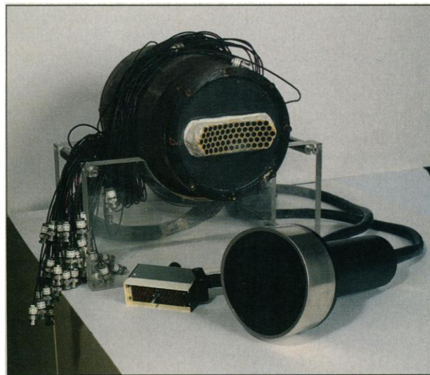
Return to sender. Mathias Fink’s “acoustic retina” takes an incoming sound wave, digitizes it, reverses it, and sends it back along its original path as if time were going backward.
