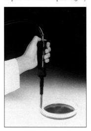
vacuum suction is required. It was designed to replace traditional glass pipettes. It works by attaching a tube from the top of the pipette to a vacuum system. The liquid is aspirated by a disposable tip through the pipettor to a waste container. The Vacupette reduces the risk of contamination
