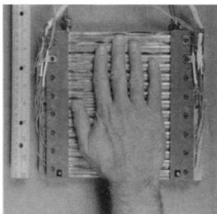
**Fig. 1.** The thermode used with human participants. The stimulus surface (20 by 14 cm) was made of 15 1-cm-wide sterling silver bars, set about 3 mm apart. Underneath each bar were three longitudinally spaced thermoelectric (Peltier) elements (1 cm<sup>2</sup>), and a thermocouple was located on top of each bar. Alternate (even- and odd-numbered) bars could be controlled independently.
