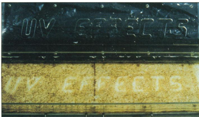
Spelling it out. Algae growth is inhibited where UV light is let in ( let-ters ), but will eventually rebound where UV-B light kills insect larvae.
