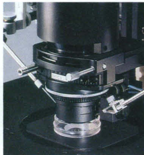
0.85 and 1.4 N.A. DIC condensers for high resolution, high magnification microscopy.
