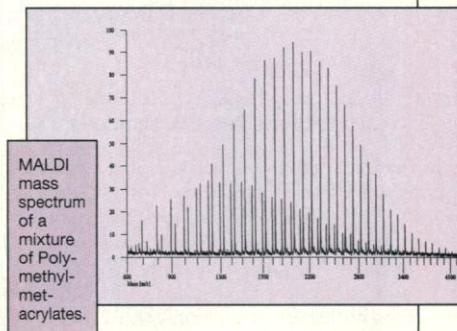
The MALDI spectrum of a polymer distribution will not only allow you to calculate  $M_w$ ,  $M_n$  and  $M_p$  from a single measurement, but it will also indicate the repeating unit as well as the end group of the polymer.
