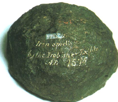
An iron bloom deposited in the Smithsonian Institution by Charles Francis Hall. "Attempts to date the bloom . . . led to the current interest in the Frobisher voyages and the Meta Incognita Program." Diameter, about 18 centimeters at base. [From Archeology of the Frobisher Voyages ]
