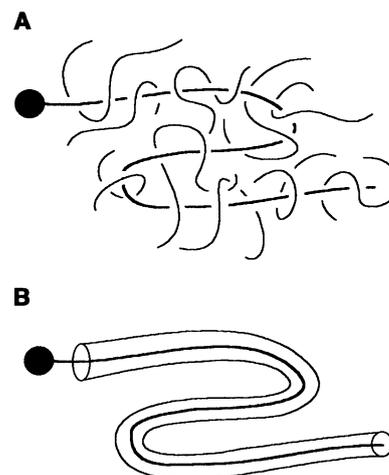
**Fig. 1.** Schematic representation of the experiment. (A) A stained DNA molecule in a concentrated solution of unstained  $\lambda$ -phage DNA was manipulated with optical tweezers by means of a 1.0- $\mu\text{m}$  latex bead attached to one end of the molecule. (B) The topological constraints of all the background chains collectively act to confine the polymer to motion within a tube-like region along its own contour.
