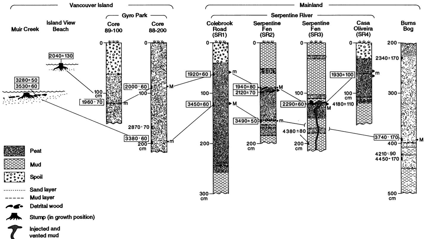
**Fig. 2.** Stratigraphic sections and correlations of two inferred earthquakes  $\sim 3400$  and  $\sim 2000$   $^{14}\text{C}$  years ago. The left side of each section is labeled with the depth (in centimeters) and the radiocarbon age (in  $^{14}\text{C}$  years before present). Symbols on the right side indicate microfossil changes at
