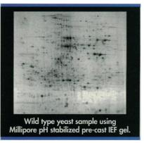
Millipore pH stabilized IEF gels are conveniently pre-cast in patented threaded alass tubes. Ready-to-use, they don't require rehydrating, cooling or messy oil overlays. And, they are compatible with any system that will accept a 1 mm x26 cm tube gel format.
