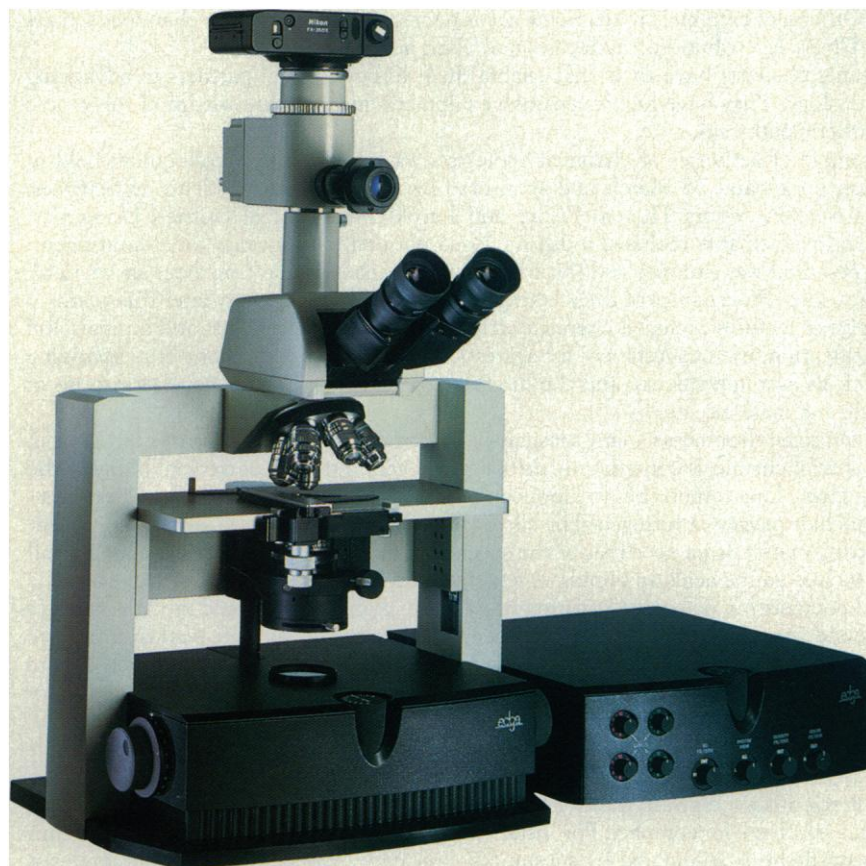
The R400 system consists of the Microscope (pictured with Nikon camera, trinocular head, and objectives), an outboard Control Box (containing lamps, filters, and control circuitry), and an outboard power supply (not pictured). Four fiber optic cables deliver "cool" light.
