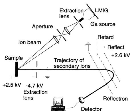
**Fig. 1.** Schematic diagram of the TOF-SIMS apparatus. Gallium ions from a liquid metal ion source (LMIG) are accelerated to 25 kV and are focused onto the sample with a spot size of  $\sim 150$  nm. The beam is pulsed by rapid electrical deflection through an aperture typically for  $\sim 20$  ns. Molecular ions sputtered from the sample are extracted through a field of 7.2 kV into a 2-m reflectron TOF analyzer. Ions are counted at a channel plate detector and processed by an online computer.
