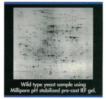
Millipore pH stabilized IEF gels are conveniently pre-cast in patented threaded glass tubes. Ready-to-use, they don't require rehydrating, cooling or messy oil overlays. And, they are compatible with any system that will accept a 1 mm x 26 cm tube gel format.
