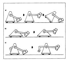
"Design problems associated with a brick-laying robot. (a) The robot is unstable once a brick is grasped. (b) Stability is achieved by altering the body shape at the expense of reduced height and increased weight. (c) Stability is achieved by the intelligent behavior of using the free arm as a counterweight." [From Intelligent Behavior in Animals and Robots]
