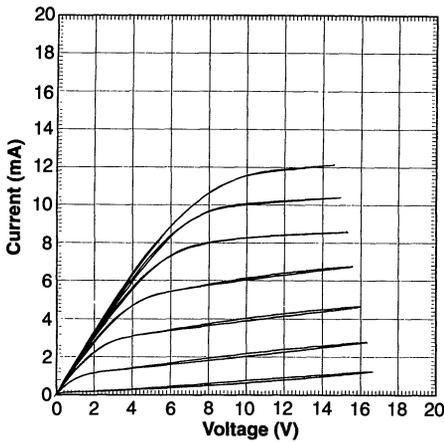
**Fig. 4.** The drain-to-source current ( $I_{DS}$ ) as a function of the drain-to-source voltage ( $V_{DS}$ ) at different gate biases ( $V_G$ , 1 V per step) for a typical GaS-GaAs FET.
