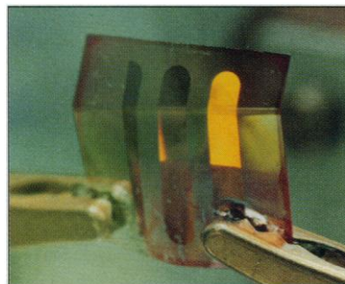
Flexible electronics. This light-emitting diode, made from PPV, a form of a conducting polymer, can be bent, a useful trait for commercial applications.
