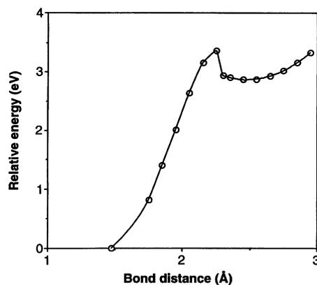
**Fig. 3.** Energetics of the triplet  $C_{60}$  window. Relative energy to the  $C_{60}$  triplet is plotted against the length of the 5-6 bond at the MNDO (UHF) level of theory. The barrier to open a bond is relatively low (3.5 eV), whereas a broad minimum exists (Fig. 1) with the bond open. This result was confirmed at ab initio levels of theory in a model system (Table 1), 5-6 bond, o.
