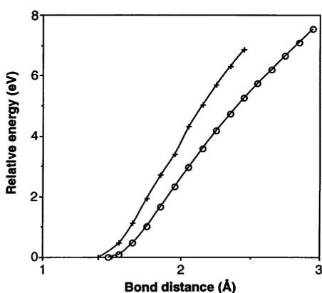
**Fig. 2.** Energetics of the singlet  $C_{60}$  bond opening. Relative energy (eV) to  $C_{60}$  is plotted against the length of the open bond at the MNDO (restricted Hartree Fock) level of theory. The 6-6 (hexagon-hexagon) bond is harder to open because it is shorter at equilibrium and has more double bond character. 6-6 bond, +; 5-6 bond, o.
