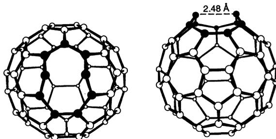
**Fig. 1.** The C<sub>60</sub> window. By breaking a pentagon-hexagon bond on C<sub>60</sub>, a large nine-membered ring is obtained. This structure with the bond open to 2.48 Å is a minimum on the MNDO unrestricted Hartree Fock (UHF) potential energy surface for the triplet state of C<sub>60</sub>.
