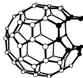
**Fig. 4.** One of several possible  $C_{60}$  "double windows." Breaking two pentagon-hexagon bonds creates a 13-membered ring in the cage structure through which large atoms or molecules may pass. The upper two sp carbons may bend back easily, opening the hole further.
