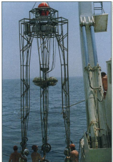
Eyes in the Aegean. Workers lower one stage of NESTOR, a neutrino detector, into the water off the island of Pylos.
