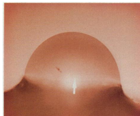
Fig. 3. Tunneling electrode made of fire-rounded Pyrex glass coated with ITO. Radius of curvature is 180 \mu\text{m} .
