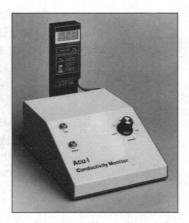
conductivity cell attaches to the eluent end of the column and digitally displays conductivity during a run. Protein tracking can be accomplished by monitoring eluent conductivity during column separations because a protein usually elutes from the column at the same conductivity value run after run. Lazar Research Laboratories. Circle 143.
