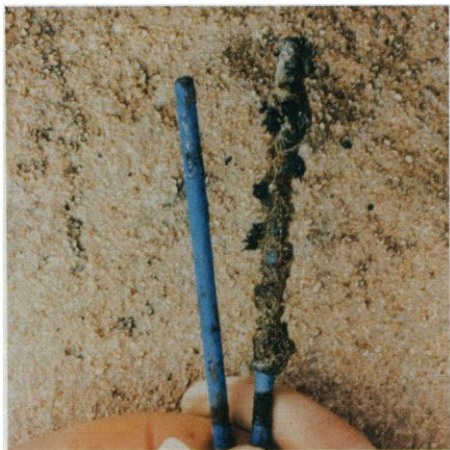
Fig. 9. Test rods from off-shore testing in Hawaii after 6 months of exposure. The rod with little fouling was coated with a paint that included tubules containing Renilla extract. The rod with the greater amount of fouling had only the base paint. [Photo by R. Price]
