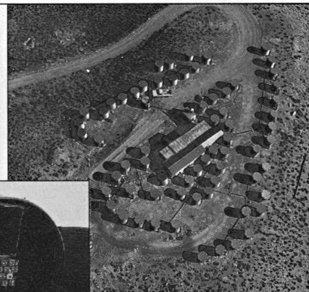
Eye on the sky. The Fly's Eye array and the photomultiplier tubes inside one detector.
