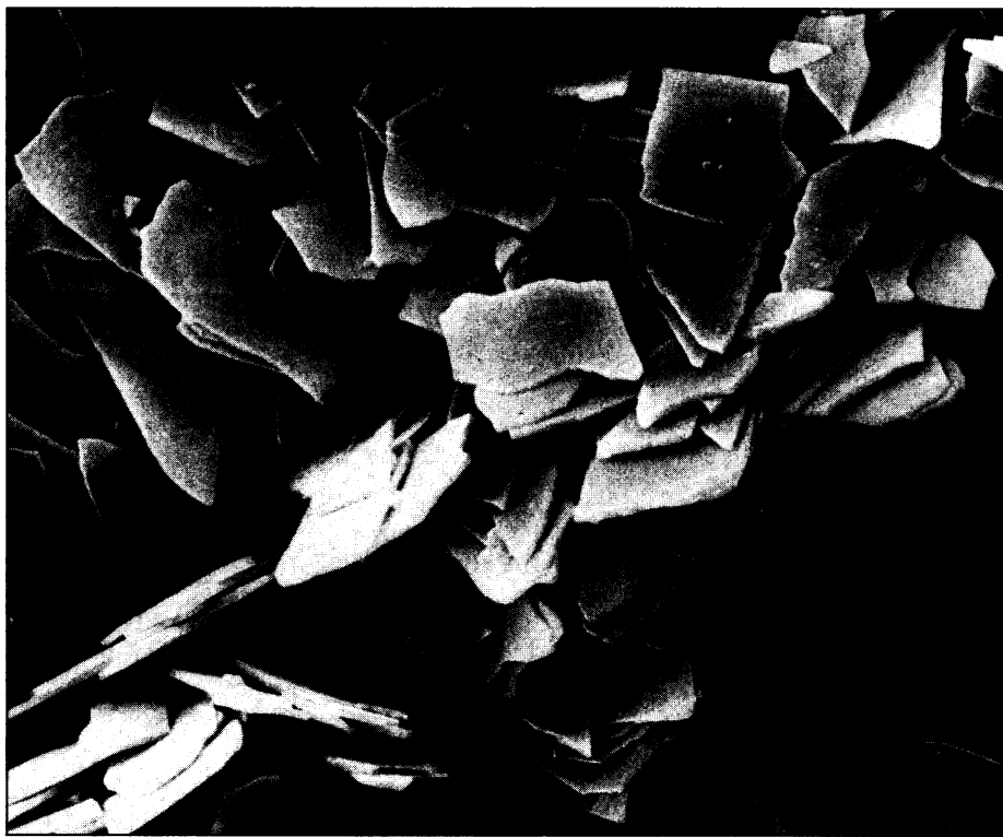
Scanning electron micrograph of the nacreous surface of the mollusk Atrina . Magnification, \times 2000 . [Courtesy of Jon Didymus, University of Bath, United Kingdom]
