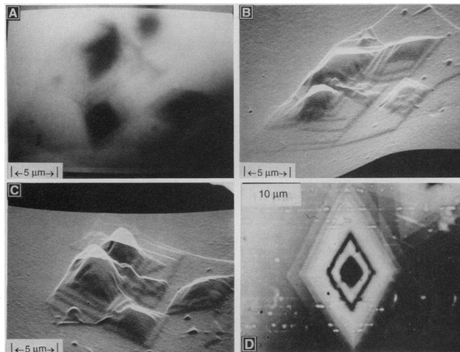
**Fig. 4.** (A) Gray-scale PTM image of single polyethylene crystals and (B and C) 3D images showing the topography from different viewpoints. (D) A single large crystal can be imaged with the PTM in contact interference mode.
