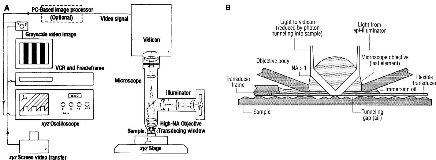
Fig. 2. Schematic diagram of (A) the photon tunneling microscope and (B) the transducer, objective, and sample.
