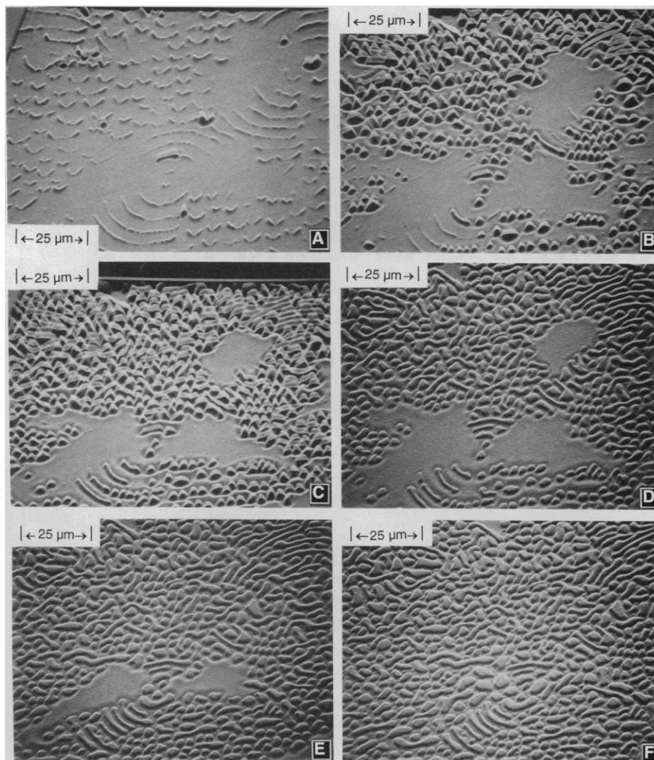
**Fig. 6.** A time sequence of the ripple structures as the polystyrene film starts to dewet: (A) 60 s, (B) 456 s, (C) 540 s, (D) 564 s, (E) 864 s, and (F) 1200 s. (C) and (D) were made almost simultaneously to show the demagnification made for clarity and to allow calibration over the entire sequence. Peak-to-valley height is typically 0.2  $\mu\text{m}$ .
