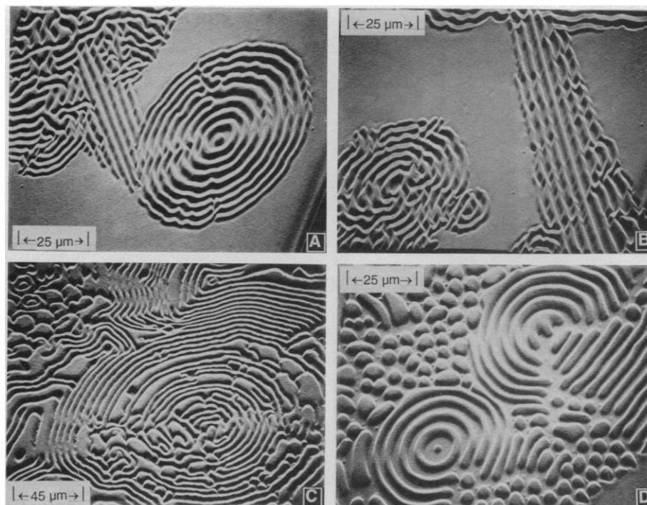
**Fig. 5.** (A through D) A selection of patterns formed during the dewetting of thin polystyrene films on a glass substrate, with a typical peak-to-valley height of 0.2  $\mu\text{m}$ . The structure shown in (C) is typical of those formed close to the contact point.
