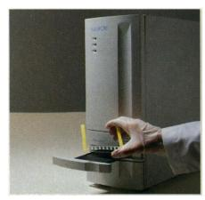
**Step 4.** Take a picture of the band pattern. Simply slide the gel cassette into the imager.
