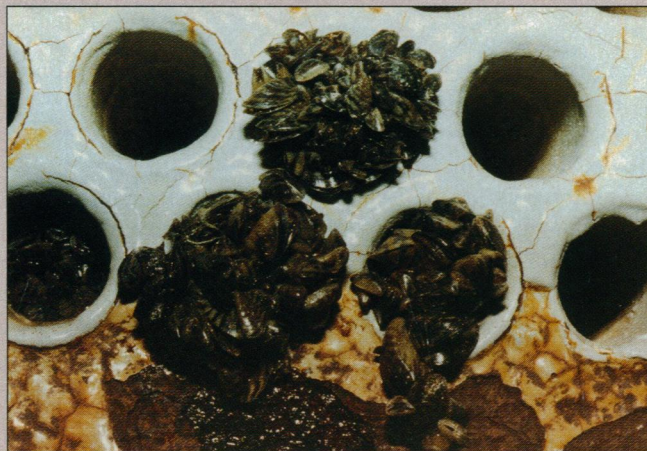
Ugh. Golfball-sized clusters of zebra mussels clog the heat exchange pipes at the Detroit Edison Co.'s Monroe Power plant in Lake Erie, Michigan.
