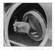
controlled environment. The design and construction of the opening eliminates the need for bulky gloves. It consists of 30 points of soft latex that conform around the wrist to prevent atmosphere exchange during use. It fits into any standard eight-inch glove box hand port. Manostat. Circle 145.
