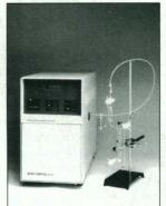
cardiovascular and neurological researchers throughout the world. Based on  $NO/O_3$  chemiluminescence, the NOA can detect < 2 picomoles of NO. An independent evaluation found that the NOA "is approximately 500 times more sensitive" than atmospheric NO monitors "for measuring nitric oxide in small volumes of solution." Special gas strip-
