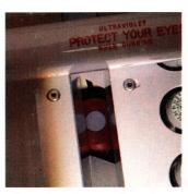
Silicon photoelectric cell monitors UV radiation in joules/cm². Together with the microprocessor control, it ensures precise exposure control and repeatability.
