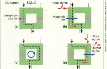
Altered states. In a SQUID—a microscopic ring of superconducting material cut by Josephson junctions—pulses of current admit and release units of magnetic flux. A high-speed signal processing device (*right*) incorporates 4096 SQUIDs.
