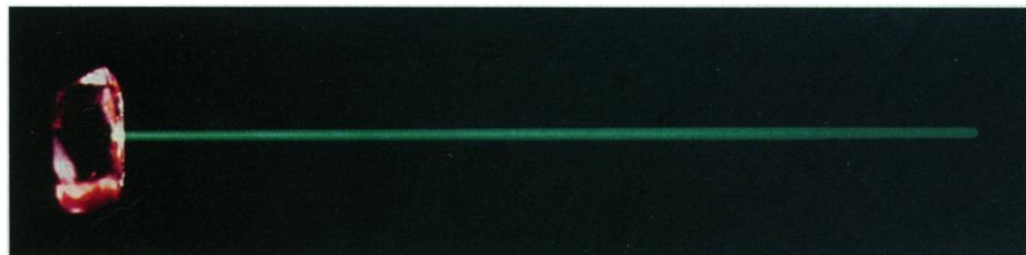
The greening of a laser. An inorganic crystal doubles the frequency of infrared laser light, an effect that materials scientists are trying to reproduce in polymers.
