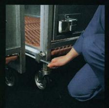
units without tools by a simple locking device, and they are quickly disassembled for very flat compact storage.
