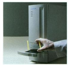
**Step 4.** Take a picture of the band pattern. Simply slide the gel cassette into the imager.
