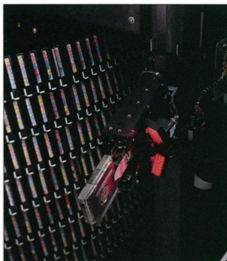
Cool hand. Robots like this Storage Technology device, which manipulates a library of 6000 tape cartridges, are likely to be used to retrieve data in EOSDIS archives.
